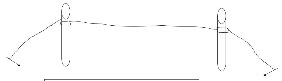
Tower / platform is 10 x 10 and 20 feet high. class 5 poles, metal stairs with 42" handrails and sides covered with expanded metal. Anchors are going east, west, north and south. safety guy wires run along 3 sides at top of poles.
