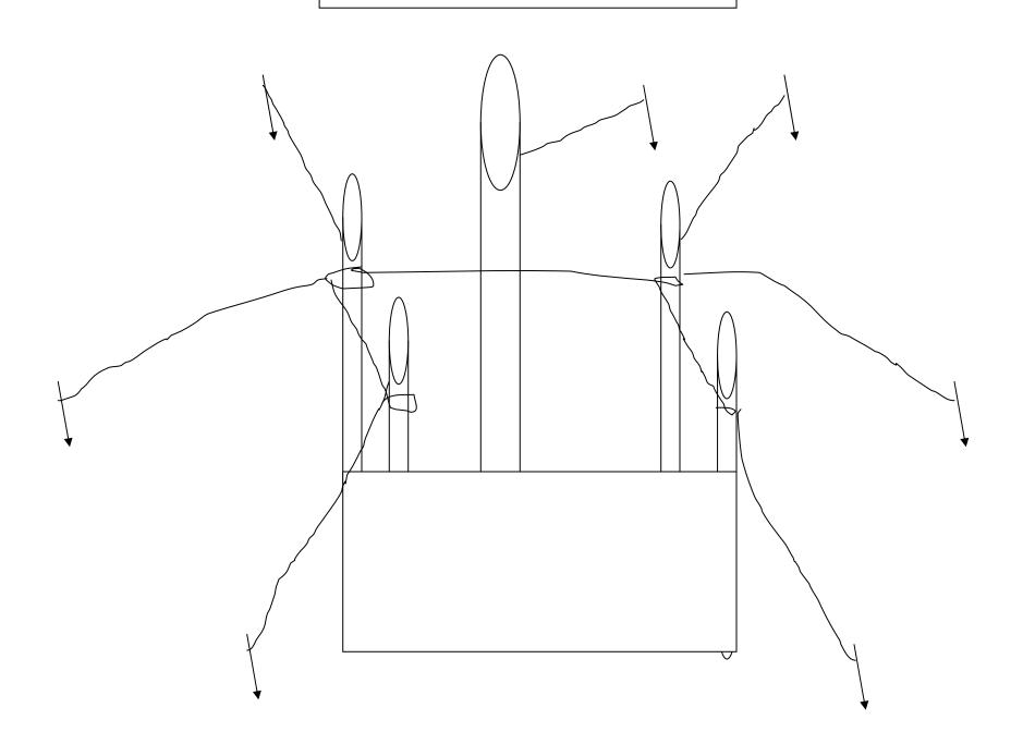
(2) class 2 poles from point A to point B. 6 feet deep and 35 foot tall. anchors are 30 feet out and 30 feet high. 5/16 wire rope (galvanized cable) with 3 u clamps at each end. zipline is 250 feet long with a 30 feet bungee block and a stop block.
