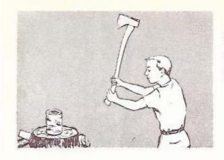
Lower the ax sharply with right hand slipping down the handle stopping just above the left hand.
