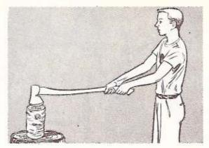
Bring the ax back to the body, grasping under the handle near the head with right hand.
